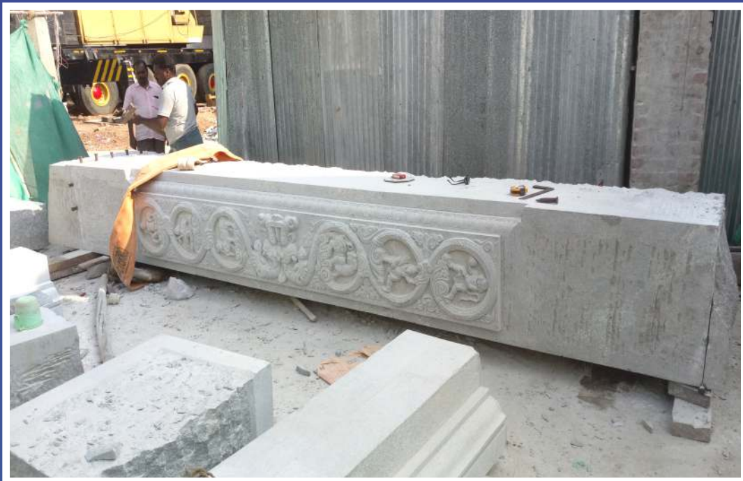
Fully carved top frame September 2018 As mined weight - 17,200 kg Finished weight - 11,200 kg
