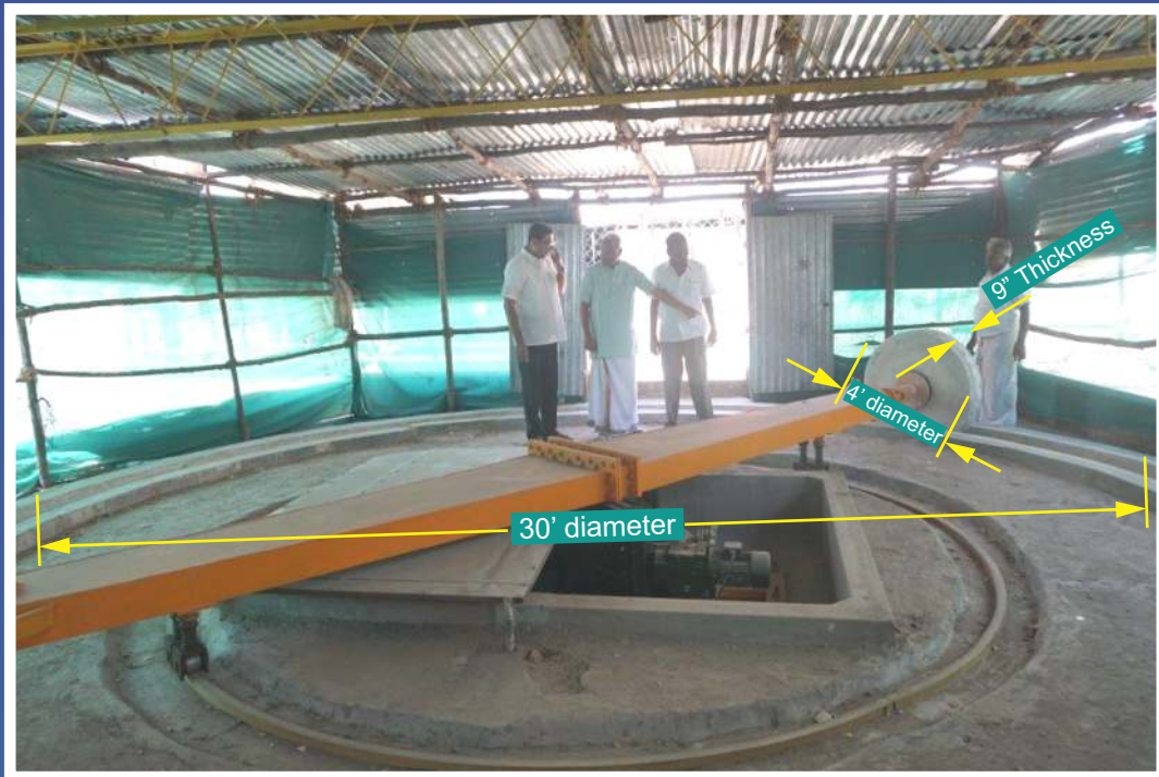
Dr. Arun Menon - IIT Consultant, Mr. V S Jayabal - Donor and Mr. Kumaragurubaran - Sthapathi discussing a Lime-Mortar mixer arrangement
